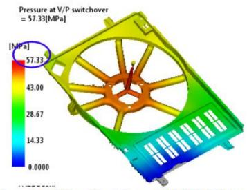
Molding Trials and Moldflow Simulation of **SHROUD** Higher Value Results. Higher Values can not be accepted. One of which can be explained here. Let us consider Maximum Pressure With PA6 is seen to be 117.6MPa and the same with PP is seen to be 57.33MPa.
