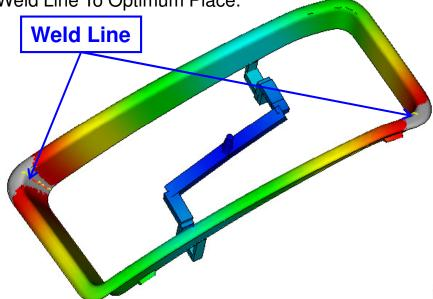
Molding Trials and Moldflow Simulation of **Chrome Were Carried Out.** Iterations Were Carried Out In Order To Shift The Weld Lines.
