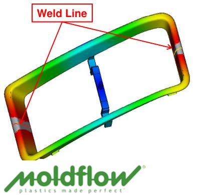
Pre Processing: Mesh Type: Dual Domain Polypropylene Material.
